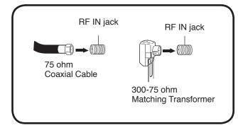
Connect the 75 ohm Cable from the Combination VHF/UHF Antenna to the RF IN Jack.
